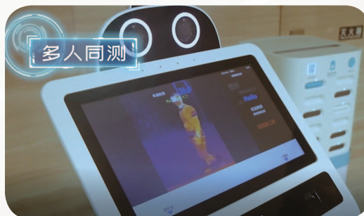
Temperature measurement robot uses infrared rapid sensing technology for temperature measurement and recognizes whether the person is wearing a mask.
