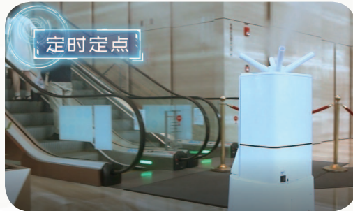
Aroma robot uses ultrasonic atomization technology to diffuse and spray fragrance at scheduled time and location
