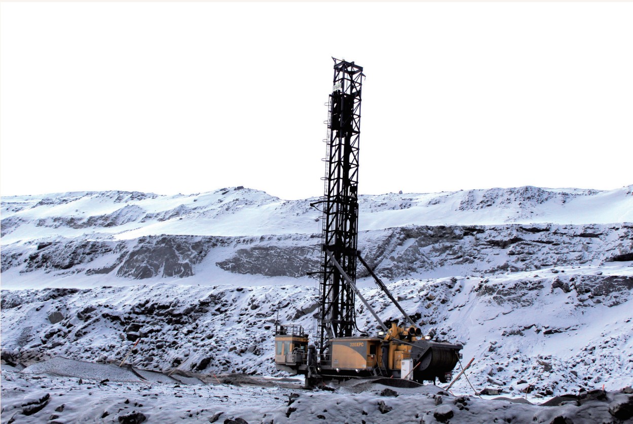
PH320 drill working on the pattern
