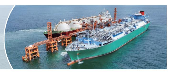
An LNG shipment (left) arrives at Hong Kong's first offshore LNG terminal, and is loaded onto the floating storage and regasification unit vessel (right), the Bauhinia Spirit, for regasification.
