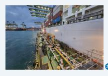
OOCL completed the first biofuel bunkering in its fleet. The fuel delivery, arranged by supplier KPI OceanConnect's team in Singapore and supplied by barge, was received by OOCL's container vessel while at port in Singapore. The B24 biofuel delivered was a blend of Used Cooking Oil Methyl Ester (UCOME) and Very Low Sulphur Fuel Oil (VLSFO).
