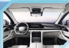
Chery Automobile powered by BOE dual 12.3" curved Mini LED instrument mid-console display
