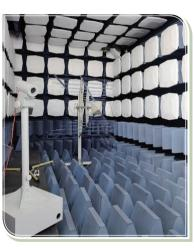
Fully Anechoic 3 meters Chamber 3米法全電波暗室
