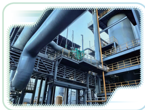
Equipment for blast furnace taking-off blast gas recycling 高爐休風放散回收設備
