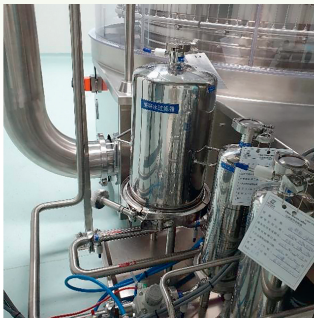
Recycled water screening procedures of a bottle washing machine
