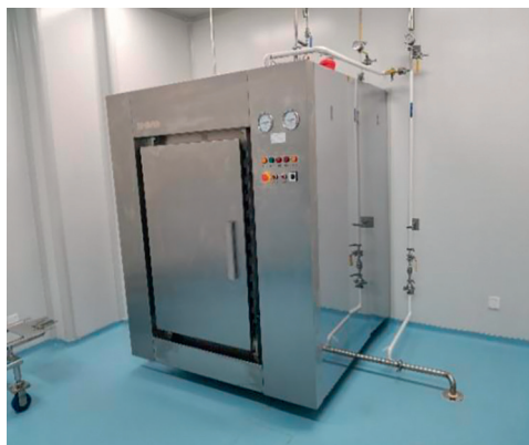
High temperature sterilization cabinet for primary slag treatment
