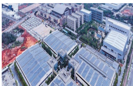
Distributed photovoltaic panels on roofs of factory buildings in Wasion Energy Industrial Park
