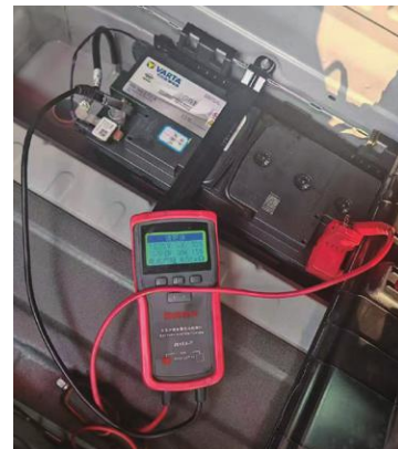
Tuhu's Automatic Battery Testing Equipment
