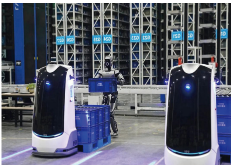
The UBTECH industrial humanoid robot Walker S1 cooperated with Wali unmanned forklift F1200S to complete the storage of automobile parts
