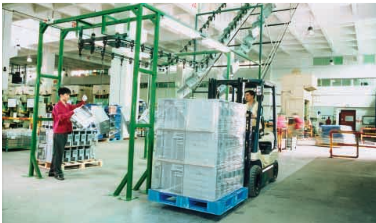
Moving semi-finished products by automatic overhead conveyor
