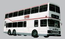
The world's first air-conditioned double-deck bus, developed by KMB, retired from KMB's bus fleet after 17 years of service. The development of this historic bus introduced a new era of double-deckers, using just one engine to control both the driveline and the air-conditioning system. The fuel savings achieved, as well as the environment-friendly design, set new benchmarks.
