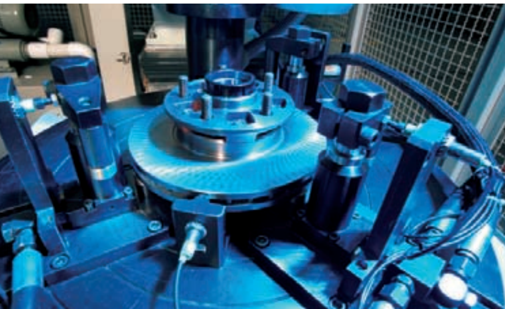
An advanced machine used to test balancing on front wheel shafts
