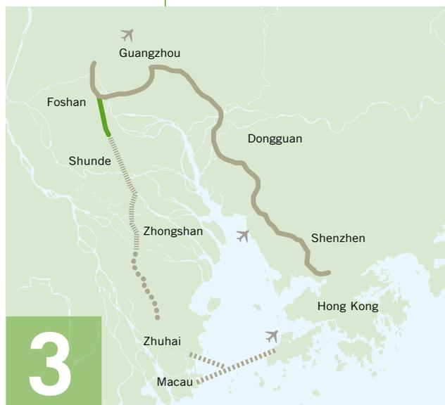
The Phase I West is a 14.7 km closed system dual three-lane expressway. It connects to the ESW Ring Road in the north and to the National Highway 105 and Bigui Road of Shunde in the south.
