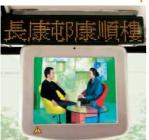
In 1998, KMB and LWB first launched the Electronic Bus Stop Announcement System which delivers voice announcements and shows the name of the upcoming bus stop on LED display on board the bus. All buses are now equipped with such systems.
