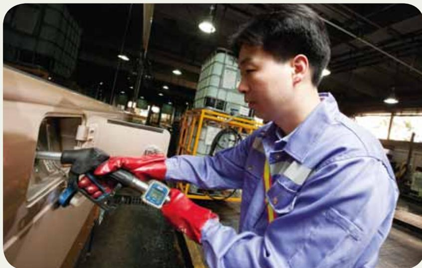
65 urea solution dispensing units have been installed across KMB's operating area
