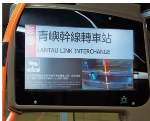
▲ Equipped with an on-board CCTV system, LWB buses display real-time footage of the luggage racks, allowing passengers to keep an eye on their belongings while seated and enjoy a comfortable, worry-free journey
