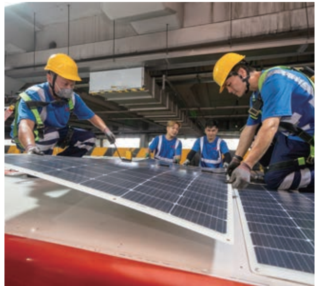
▲ KMB self-developed installation of solar films on double-decker roofs harnesses renewable energy to reduce carbon emissions
