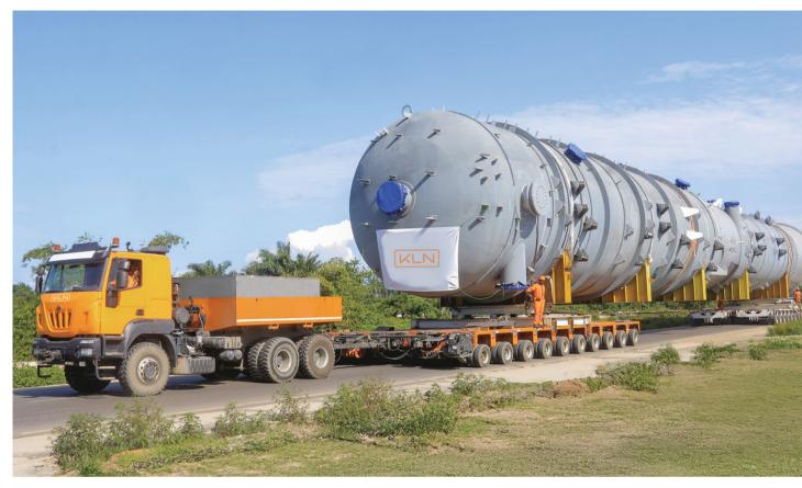
KLN Group delivered a large-scale fertiliser plant, including an ammonia converter weighing up to 643.50 tonnes, from South Korea to Nigeria via road freight between May and July 2025
