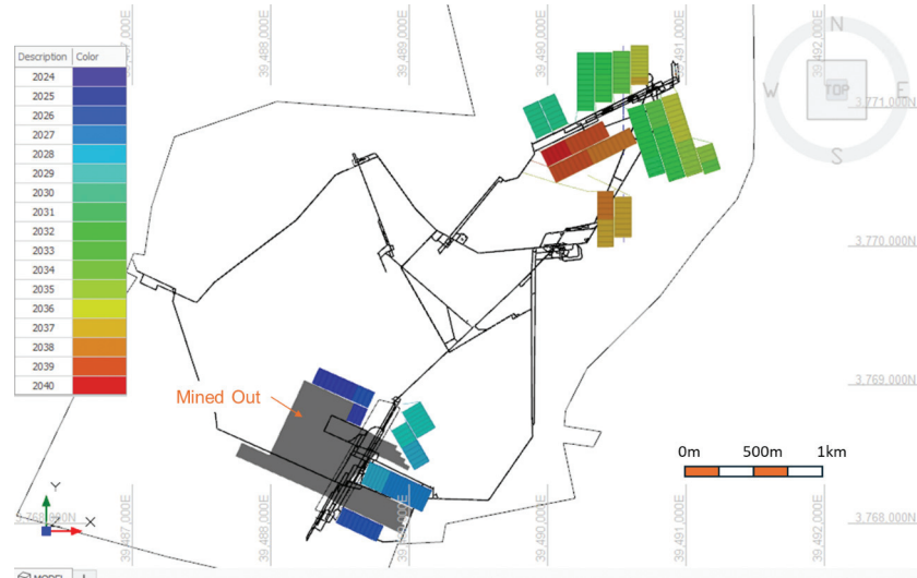
Figure 10.10: Block and panel mining sequence
