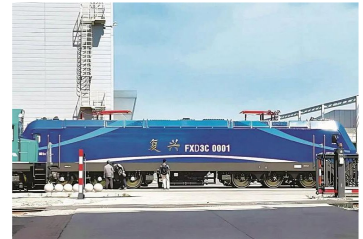
A Fuxing Locomotive Manufactured Using 100 mm Extra-thick, 460 MPa-grade-High-strength, High-toughness Steel for Locomotives
