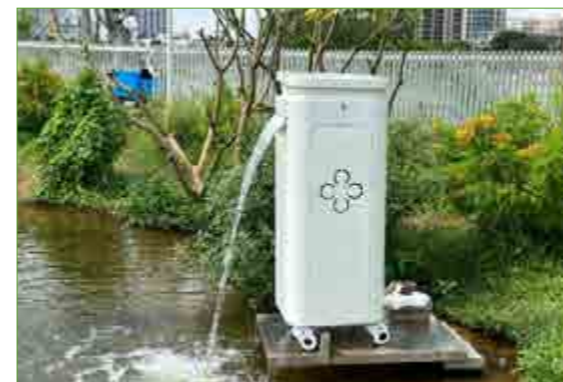
The self-developed 3D fast-filtration water quality maintenance equipment, featuring highly efficient algae and turbidity removal capabilities, together with intelligent automated surface debris collection stations capable of intelligent identification and efficient retrieval, has been deployed at scale.
