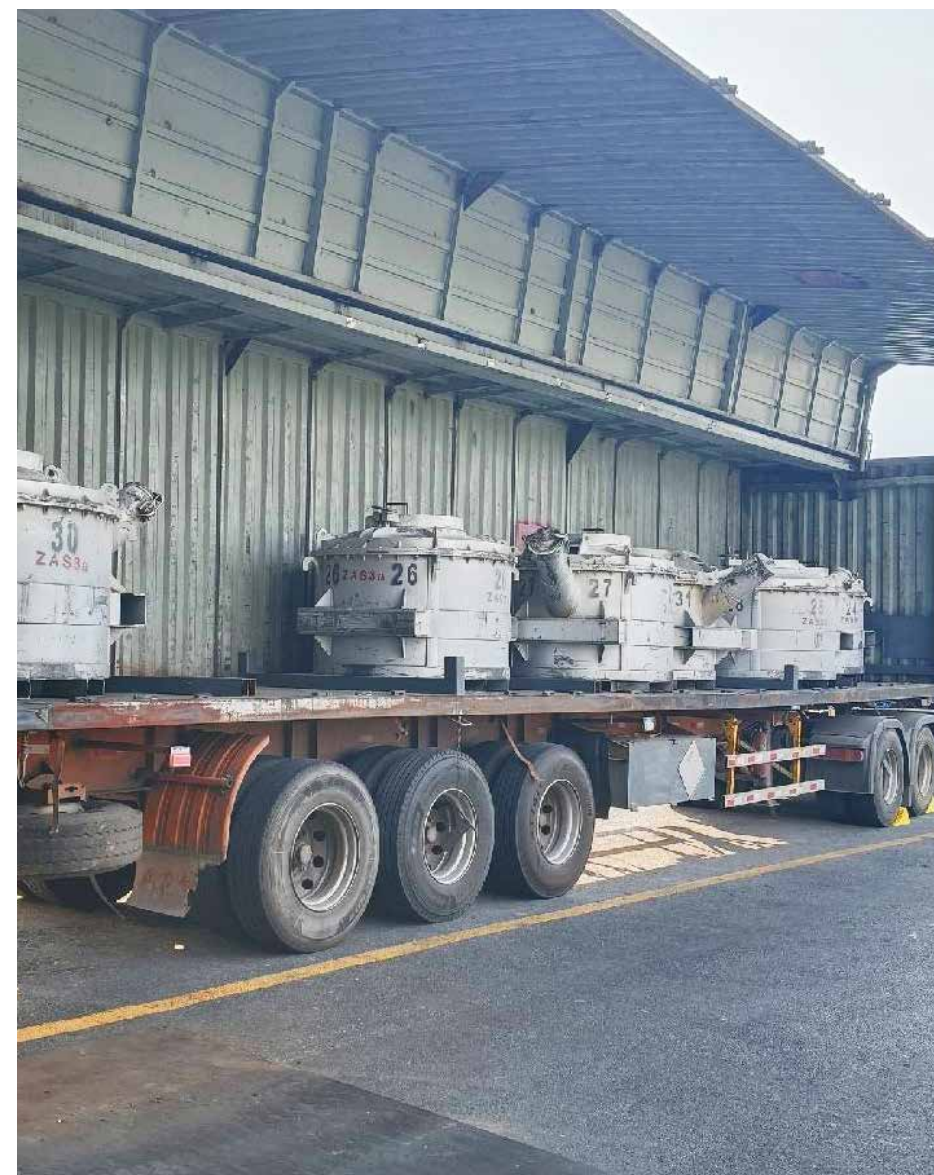
Delivery of high-temperature molten aluminum to the workshop
