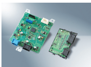
Battery management system
