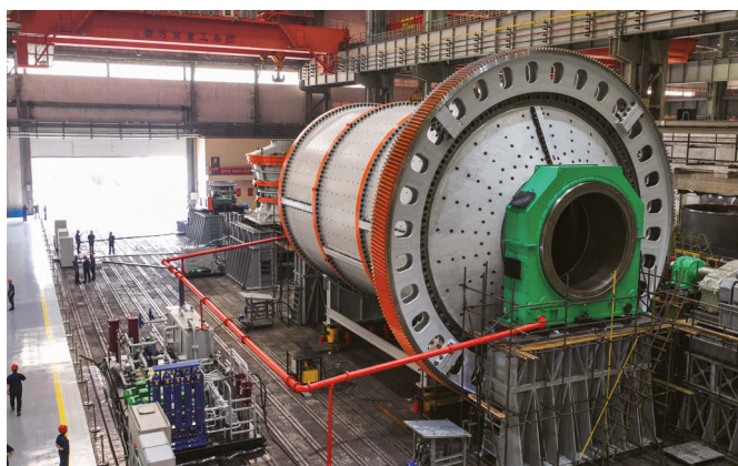
CITIC Heavy Industries has delivered the largest domestically manufactured \phi 8.2\text{m} \times 12.7\text{m} overflow ball mill for the Ghana project.
